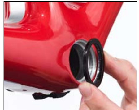
Figure 41. Inserting the bearing cups into the bottom bracket shell
